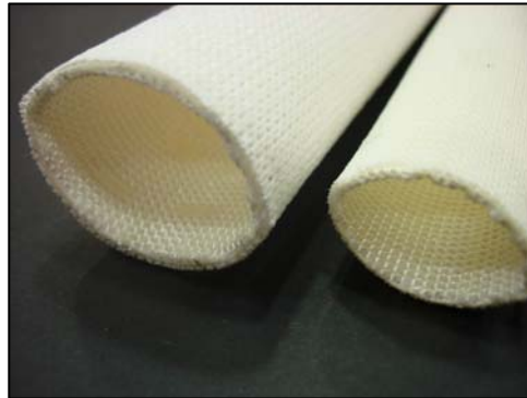
Weft circular machine with internal and external insertion of the fabric. With intermediate polyethylene coat.
