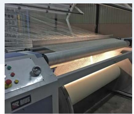
Warping machine driven by PLC and computer touch screen.
