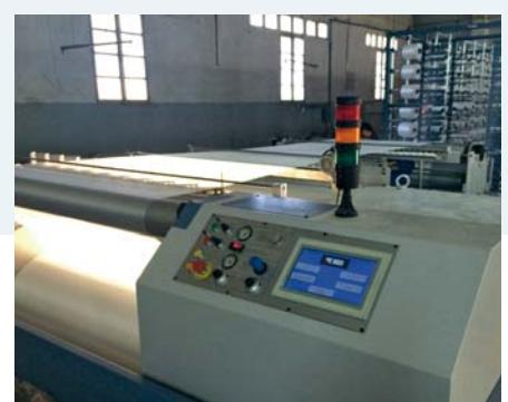
Warping machine driven by PLC and computer touch screen.
