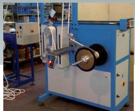
High precision semi-automatic rolling and measuring machine for large diameters cords and ropes, as well as rigid special tapes.
