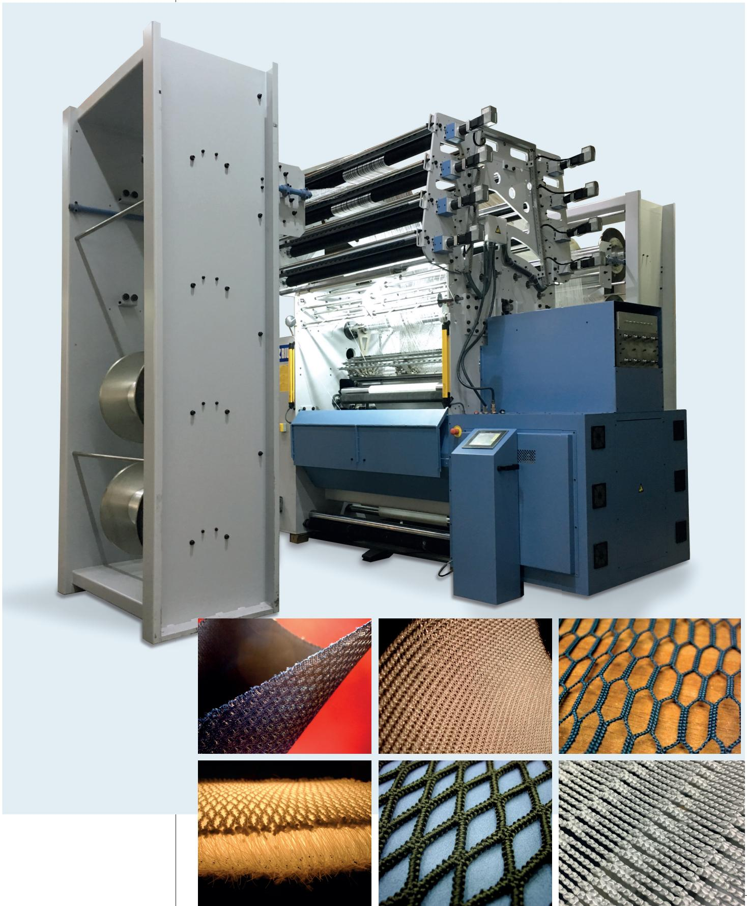
High efficiency electronic double needle bed warp knitting machine of versatile use (Raschel knitting system), for the production of flat knitted fabrics, tubular fabrics as well as technical meshes, knot-free nets and structure 3D fabrics.
