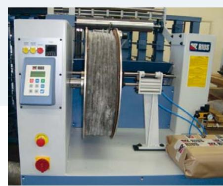
Tape spooling machine, for special spools of 750 mm. of diameter x 750 mm. width (model MTP 750).
