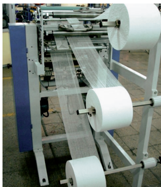
Application in our cutting and folding machines for the production of compresses.
