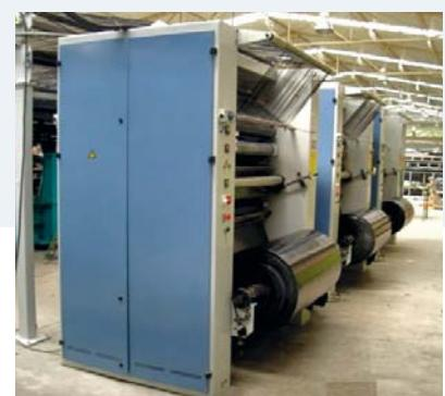
Modular cutting and stretching system from polyethylene film, to feed Raschel machines, crochet and circular warp knitting machines.
