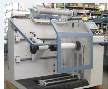
Easy handling warping machine with all functions electronically controlled.
